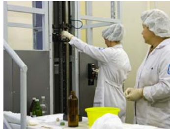
Coating clean room. Left to right: long tubes coating; on the wall - humidity control unit, on the right – primary drying chamber, in the center – secondary drying chamber and final open drying. The cycle takes up to seven days
