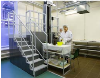
Coating clean room. Left to right: long tubes coating; on the wall - humidity control unit, on the right – primary drying chamber, in the center – secondary drying chamber and final open drying. The cycle takes up to seven days
