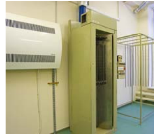
Coating clean room. Left to right: long tubes coating; on the wall - humidity control unit, on the right – primary drying chamber, in the center – secondary drying chamber and final open drying. The cycle takes up to seven days
