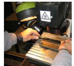
Laser engraving: brand, cat. number, s/n, lot number, dates: private labeling option and full traceability. Last step before packaging
