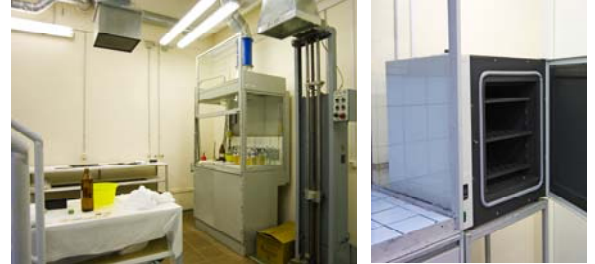
Coating clean room: solution preparation chamber, stand for coating shorter tubes, chamber for THF preparation
