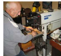
Laser engraving: brand, cat. number, s/n, lot number, dates: private labeling option and full traceability. Last step before packaging
